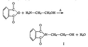
A study of the oxidation of  $\beta$ -hydroxyethylphthalimide (I) to phthalylglycine (II) was made and found to give an 89–93% yield of crude material when acidified potassium dichromate was used as the oxidizing agent.
